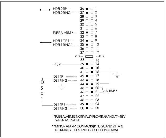
Figure 5. HLU-231, List 6 Pin-Outs. The active pins are highlighted in black in the above illustration.
