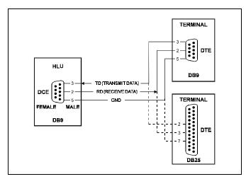
**Figure 3. HLU-231, List 6 DB-9 Pin-Outs.** A standard RS-232 (DB-9) connector on the front panel provides access to the menu interface feature via a dumb terminal.
