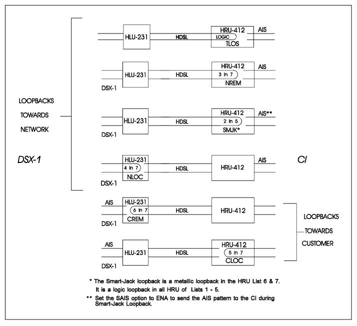
**Figure 4. HLU-231 Loopback Configurations.** The most important of the HiGain family of loopback options is the Smart-Jack loopback, which emulates the functions of a standard NID.
