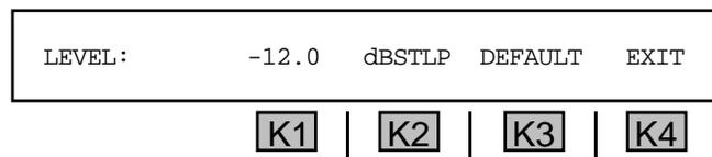
5. Use the **numeric keypad** to enter a new level, and then press **K4** to exit to the **MODIFY** display.
