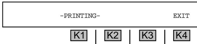
2. Press **K4** under **EXIT** to abort printing. When all records have been printed, the **930A** returns to the main **SETUP** display.
