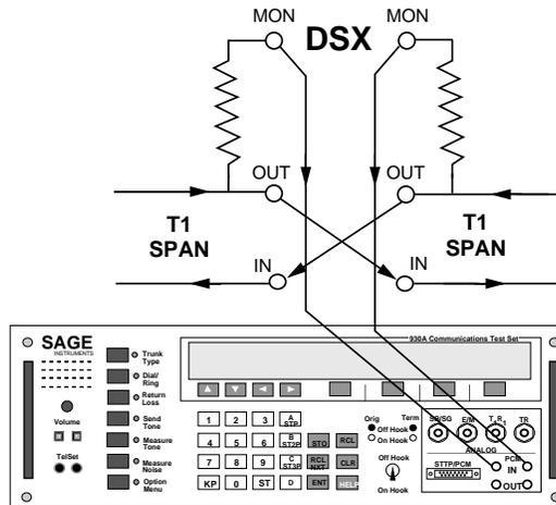
The 930A must be set to 100 Ohms Impedance and placed in the MON 1&2 mode.
