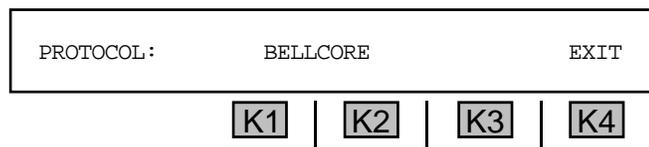
2. Press **K1** or **K2** under **BELLCORE** to scroll through available protocols.
