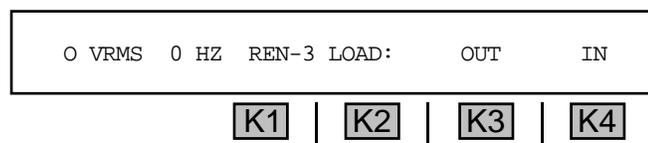
5. Press **K3** under **OUT** to place the **REN-3** Load off-line (as shown above), **OR** press **K4** under **IN** to have the **930A** act as a true **REN-3** Load at its **TR** or **T1R1** jacks.
