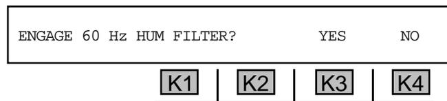
4. Press **K3** under **YES** to engage a **HUM** filter, **OR K4** under **NO** to disengage the filter.
