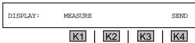
2. Press **K4** under **SEND** if you want to display what you are sending, **OR** press **K2** under **MEASURE** if you require a measurement. The measure function will display the measured frequency as you sweep on the transmit. The display reads:
