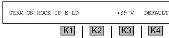
The **930A** will provide no supervision indication if the voltage on the **'E'** lead is below the high threshold of **39 V** but above the low threshold of **11 V**. The high threshold can be changed to **20 V** as before.
