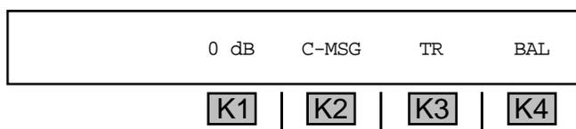
2. Press **K2** to scroll through the weighting filters: **3K FLT** (3 kHz Flat), **C-MSG** (C-Message), **C-NOTCH**, or **S/N** (Signal-to-Noise). In Wideband, **15K FLT** (15 kHz Flat), **PROGRAM**, **50 K-BIT** and **E-FILTER** are also available filters. The **DSL** and **HDSL** technologies require a flat response out to approximately **100 kHz** using the **E-FILTER**.
