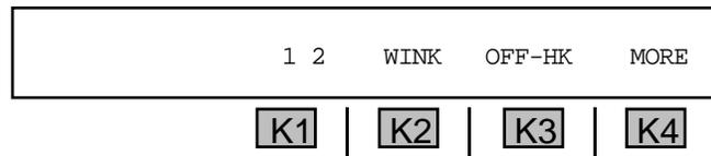
10. Go **off-hook**. The numbers stored in the two registers will be automatically outpulsed as a single digit string with a pause between the two records (approx. 1 sec)
