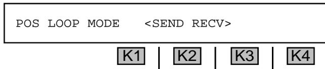
1. Use the **Up/Down Arrow** keys to scroll through the customer states: POS (positive) LOOP MODE, GROUND START, POS COIN CHK, -R RINGING, POS COIN CTRL, NEG COIN CTRL, NEG COIN CHK, NEG LOOP MODE, or CHANNEL TEST.
