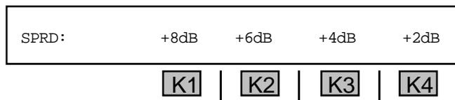
**8 dB spread is not available with thresholds above 96 dBrnC.**
