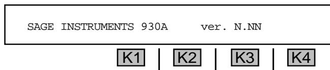
**N.NN** is the version of software installed in the unit. Note the status of the LEDs on the front panel. If an error has been detected, all of the LEDs will be lit. Turn the **930A** off and perform a cold boot.
