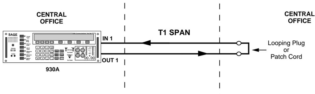
Use the factory defaults for testing if the far-end is looped back.
