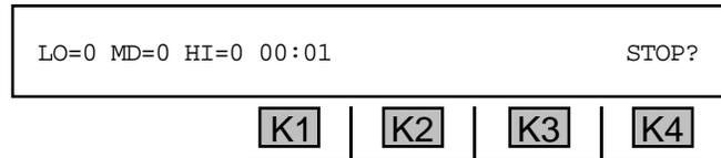
If you need to stop the test, press **K4** under **STOP**. Otherwise the test will accumulate impulse noise as selected under the **TEST LENGTH** display.
