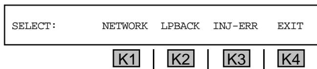
**LPBACK** is displayed above **K2** in all modes except **64KB** mode. **NETWORK** is displayed above **K1** in **DS0A** and **DS0B** only. This allows access to the network configuration code (**NET-CODE**) displays and the multiport junction unit (**MJU**) configuration displays.
