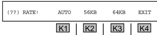
12. Press **K1** to select **AUTO** data rate detect, **K2** to select **56KB** rate detect, or **K3** to select **64KB** rate detect. You will advance to the **IMPEDANCE** display:
