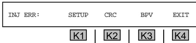
2. Press the softkey (**K1-K4**) beneath the type of error you want the **930A** to send. To inject a Bipolar Violation, press **K3** under **BPV**. To inject a **FRAME** error in **D4/SF**, or a **CRC** error in **ESF**, press **K2**.
