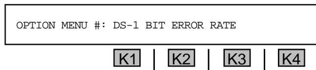
5. Press **ENT** or any softkey (**K1-K4**) to activate your selection. If the **930A** is not in **PCM** mode, the display will momentarily read **SETTING T-1 MODE . . . STAND BY**. (Refer to **Section 4, PCM Operation** for more information.)
