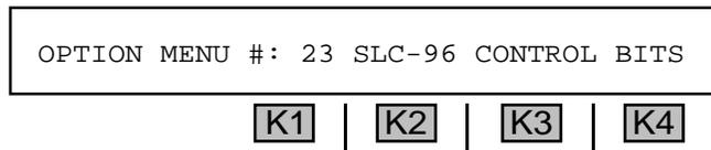
4. Press **ENT** or any softkey (**K1-K4**) to activate your selection. If the **930A** is not in **SLC-96** mode, the display reads: **MUST BE IN PCM WITH SLC-96 FRAMING**. Otherwise, you will see the displays shown on the following pages.
