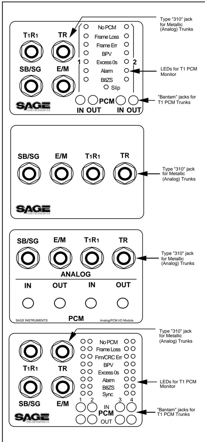
The **LED Configurator** is the standard configurator for **PCM** units. LEDs indicate status and errors on the 2 **T1** lines (**PCM1** & **PCM2**).
