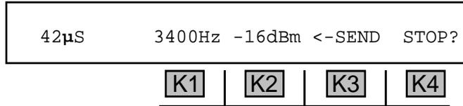
When the sweep completes or is interrupted, the **930A** will revert to sending the reference frequency. **K4** will again be labeled **SWEEP**. The sweep can be repeated or the frequency of the signal can be manually set to examine the delay at frequencies of interest.
