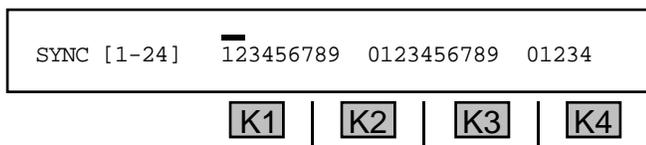
The display above shows the synchronization status for up to 24 channels on the T1 under test. A number with no line above it indicates that the indicated channel is synchronized, while a number with a line above it indicates that the channel is not synchronized.. A - indicated that the channel is not enabled.
