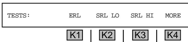
15. Press the softkey (**K1-K4**) directly beneath a return loss measurement to select or deselect it.
