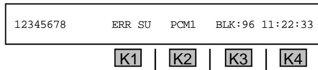
The status field above **K1** displays the error type. The following is a list of error types:
