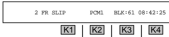
The above display shows the 61st 15-minute block of time since the test began (roughly 15 hours).
