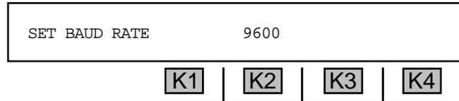
2. Use the **numeric keypad** to enter a new baud rate.
