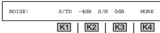
The Signal-to-Total-Distortion Ratio (**S/TD**) is displayed above **K2**, and the Signal-to-Noise Ratio (**S/N**) is displayed above **K3**.
