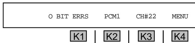
2. Press **K1** or use the **Up/Down Arrow** keys to scroll through the following tests/ results:
