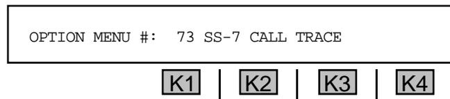
3. Press **ENT** or any softkey (**K1-K4**) to enter the **SELECT** display. The display reads:
