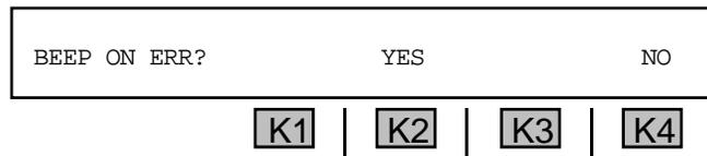
4. Press **K4** under **NO** to turn the beep **off**, **OR** press **K2** under **YES** to turn the beep **on**.
