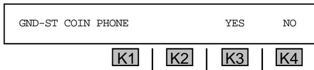
5. Press **K2** under **YES** to put the **930A** in the coin phone mode. The **930A** functions and menu options continue to operate as usual.
