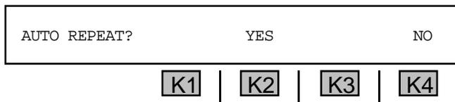
7. Press **K2** under **YES** if you wish the test to continuously repeat, **OR** press **K4** under **NO** to send the sequence only once. The display reads:
