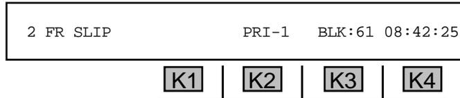
The above display shows the 61st 15-minute block of time since the test began.
