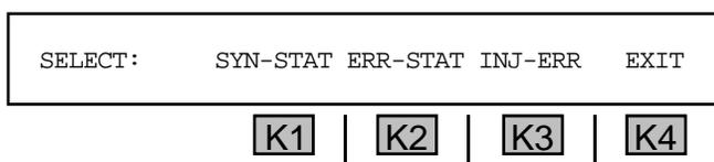
2. Press **K1** under **SYN-STAT** to view the synchronization status, **OR** **K2** under **ERR-STAT** to view the error results.
