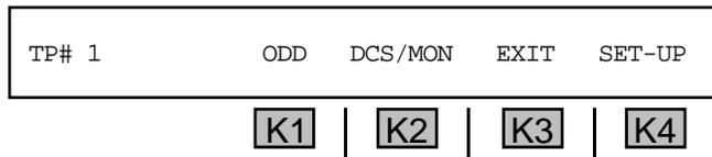
5. Use the **Up/Down Arrow** keys to scroll through the test port numbers (**TP#**).
