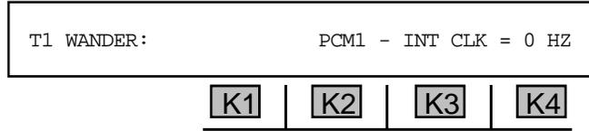
In this case the **930A** compares the clock on **PCM IN 1** to its own **Internal Clock**. Do not expect **PCM1** to agree with the **Internal Clock**, unless the far-end is Loop-Timed to the **930A**. The actual value is not significant. Large changes in the readings, however, indicate that the clock in your switch, or the clock in your **930A**, is wandering and needs to be repaired.
