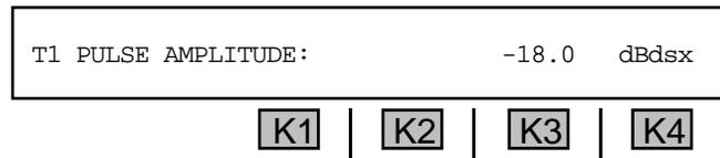
**3.0** volts base-to-peak is equal to **0.0 dBdsx**. Readings between **-1.0** and **1.0 dBdsx** would be expected at the **DSX** output jacks. Readings of about **-20 dBdsx** would be expected at the **DSX** monitor jacks.
