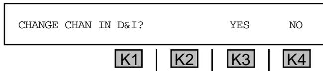
5. Press **K3** under **YES** to change the channel and leave the unit in **D&I**, **OR** press **K4** under **NO** for no change. You will be returned to the previous display.
