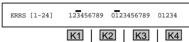
The display above shows the error status for up to 24 channels on the T1 under test. A number with no line above it indicates the absence of an error or errors on the indicated channel, while a number with a line above it indicates the presence of an error. A . indicated that the channel is not enabled.
