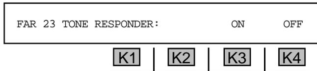
3. Press **K3** under **ON** to set up the **930A** as a 23 tone far end responder, **OR** **K4** under **OFF** to deactivate the responder function.
