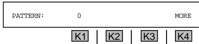
You can use the **numeric keypad** to enter any 8 bit pattern of 1s and 0s and then press **K4** under **MORE** when complete. You will be returned to the main **SELECT** display.
