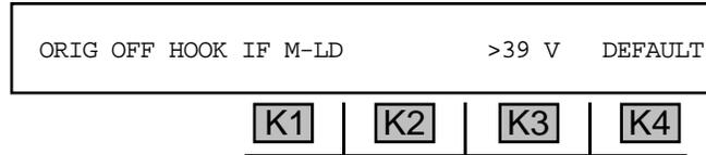
In this case the **930A** will provide an **Off Hook** indication on the **ORIG LEDs** if the voltage on the **'M'** lead exceeds the **39 V** threshold. This value has to be changed to **20 V** (roughly half of 39).
