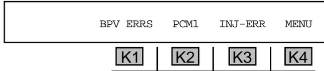
2. Press **K2** under **PCM1** to toggle between sides 1 and 2. If side 2 is not connected, you will see **NO PCM**. If side 2 is connected, the test results for **PCM2** will be displayed above **K1**.
