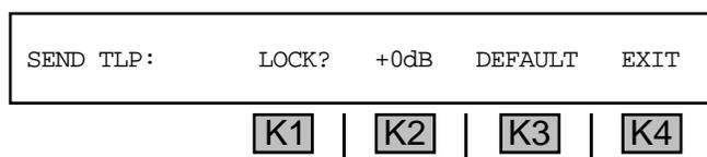
5. Use the **numeric keypad** to enter a new **TLP** (the **D** key will change the value from **+** to **-**).
