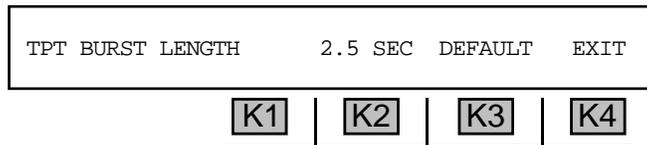
4. Use the **numeric keypad** to enter the burst length.
