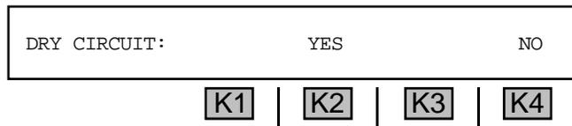
4. Press **K2** under **YES** to bring **930A** to **Dry Circuit** mode. The display reads:
