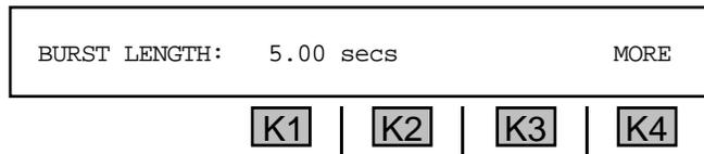
Use the **numeric keypad** to enter a new **burst length**.
