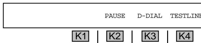
6. Press **K2** to add a - (one-second pause) to your sequence, **K3** to add a D (dial delay), **OR** press **K4** to select a testline.
