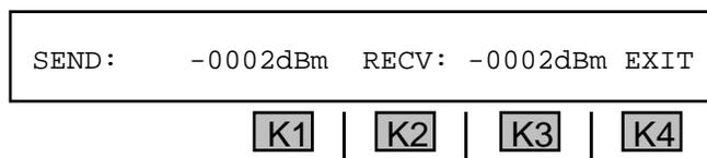
7. Press **K1** to change the **SEND TLP** or **K3** to change the **RECV TLP**.
