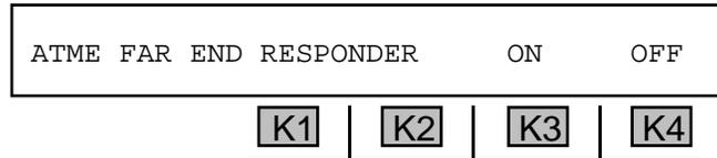
11. Press **K3** to enable the Far End Responder. A cursor will appear over the **ON** indication. The **930A** is now acting as an ATME Responder waiting to be accessed. The above display appears regardless of whether or not the **930A** is in manual sequence mode.
