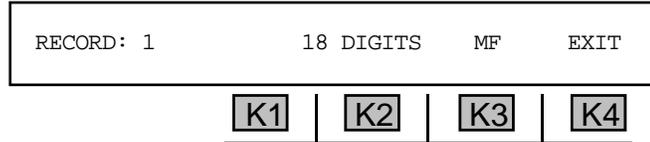
2. Press **K3** to select the signalling type. The display cycles between **MF** (Multi-Frequency) **DTMF** (Touchtone®), or **DP** (Dial Pulse).
