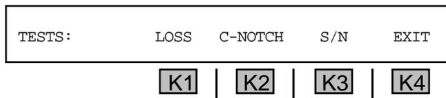
6. Press the softkey (**K1-K4**) beneath a test to select or deselect it. **LOSS** tests are performed at **1004 Hz**. **C-NOTCH** measures C-Notch noise. **S/N** measures a **1004 Hz** signal-to-noise ratio. The default parameters will show all tests to be selected.
