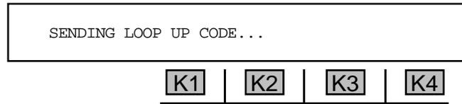
When the loop-up is completed, the display reads: **REMOTE LOOP UP ESTABLISHED**. If the loop-up is not successful the display reads: **REMOTE LOOP UP UNSUCCESSFUL** and you will return to the main **BERT** display.
