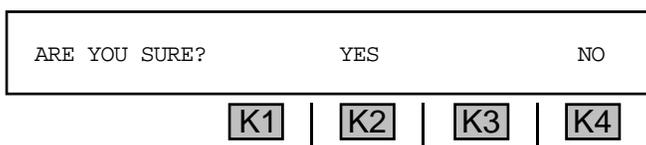
3. Press **K4** under **NO** to return to the current mode **OR** press **K2** under **YES** to activate **TERMINATE** or **MON-1**.
