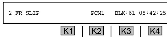
The above display shows the 61st 15-minute block of time since the test began.
