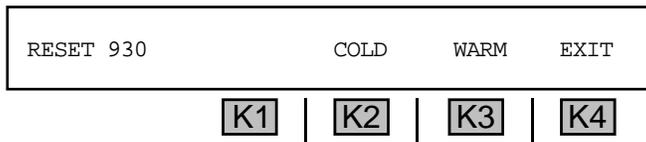
4. Press **K2** under **COLD** to cold-boot **OR** press **K3** under **WARM** to warm boot.
