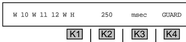
A flashing cursor will appear over the last completed wink (**w**) or off-hook (**H**) in the sequence. If a wink or off-hook has failed, the cursor will appear over the failed event. If the sequence has not yet been outpulsed, the cursor will appear over the first supervision event and all measurements will be zero.
