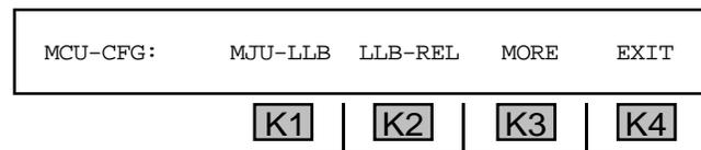
2. Press **K1** to send the latched loopback command. The display reads: **MJU-LLB: SENDING LOOPBACK CODE...**
