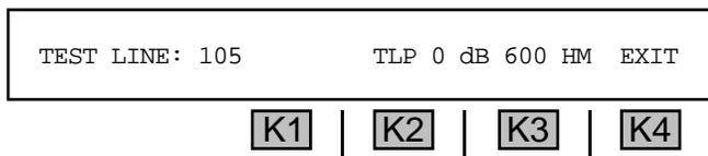
9. Press **K1** to scroll through the **TEST LINE** options of 100, 102, and 105. 105 is the default.
