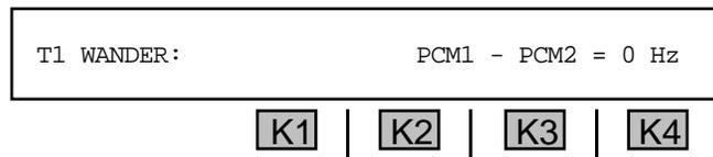
In this case, the **930A** compares the clock on **PCM IN 1** with the clock on **PCM IN 2**. Note the sign on the result. If **PCM2** is higher, the sign will be (-)
