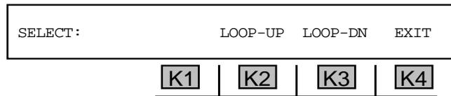
15. Press **K3** to send loop-down sequence. If you selected **sw56** testing, only **V.54** is a valid loop code. If you selected an **ALB** code, the display will read **LOOP CODES STOPPED...** If you selected an **LLB** code or **DS0DP** code, the display will read **SENDING LOOP DOWN CODE...**
