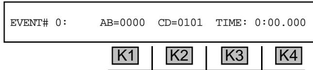
**EVENT # 0:** will always display first; this is usually an on-hook state for **metallic** trunk types. In **PCM**, the individual **A, B, C, D**, states are displayed whether on or off hook.
