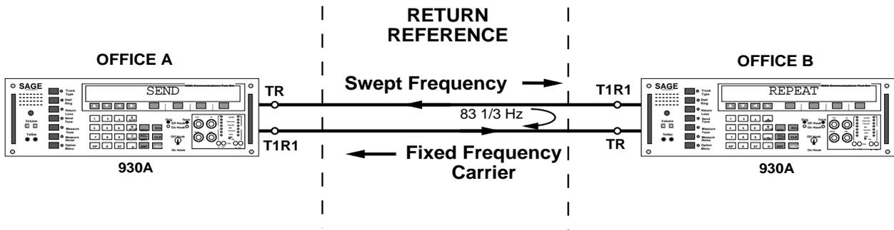
1. Office A sends an amplitude-modulated signal over the trunk under test.
