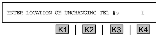
3. Use the **numeric keypad** to enter the number of the memory location where the telephone number is stored.
