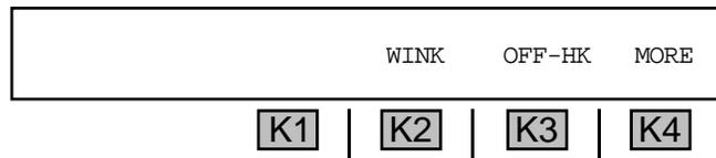
2. Press **K2** under **WINK** to add a **w** (wink) to your sequence (for a Wink Start trunk), **OR** press **K3** under **OFF-HK** to add an **H** (off-hook) (for a Ground Start trunk in **TERM** mode. )
