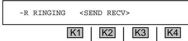
1. Use the **Up/Down Arrow** keys to scroll through the customer states: **-R RINGING**, **IDLE**, **GROUND START**, or **CHANNEL TEST**.
