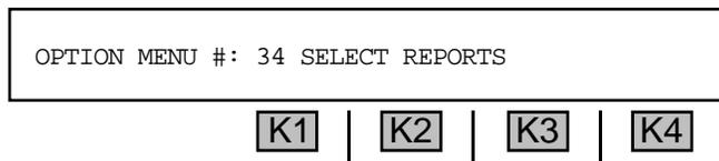
3. Press **ENT** or any softkey (**K1-K4**) to activate your selection. If you are in **COMPUTER** or **TERMINAL** remote mode, the display reads:
