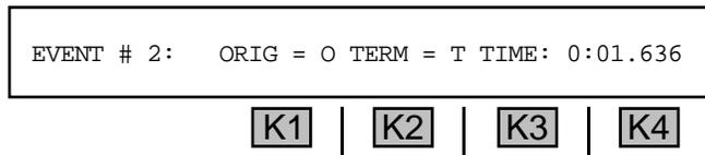
Here, the **TERM** end has gone off-hook (uppercase **'T'**) after **1.636 seconds**. The **930A** can time up to **200 events** for up to **4 hours** unless a printer is connected. In this case the **930A** continuously dumps its buffer when full and records continuously.
