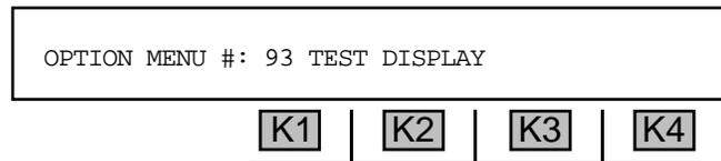
3. Press **ENT** or any softkey (**K1-K4**) and all lights and LEDs will go on.
