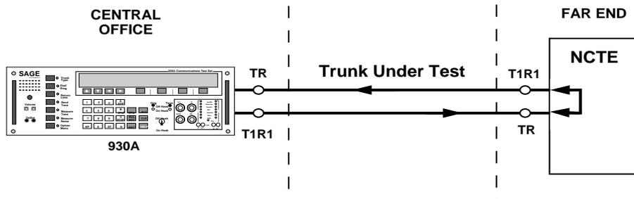
Test setup between two COs with far end looped back
