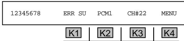
2. Press the **Up/Down Arrow** keys to scroll through the error results shown on the far left of the display.
