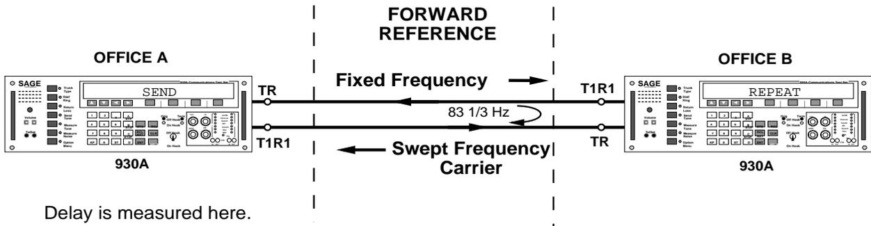
To use the **envelope delay distortion measurement function**:
