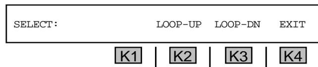
11. Press **K2** for **LOOP-UP** function. The display reads:
