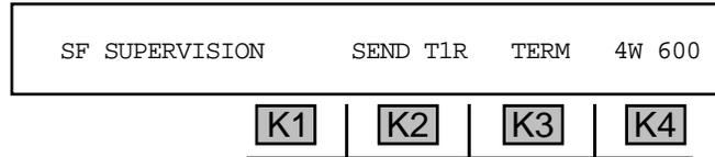
4. Press **K2** to toggle between sending on Tip/Ring (**SEND TR**) **OR** sending on Tip1/Ring1 (**SEND T1R1**).
