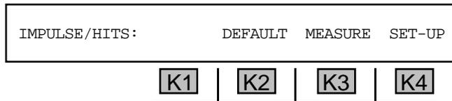
4. Press **K2** under **DEFAULT** to set the **930A** to **4 dB** spread and **7** measurements per second. The **930A** will display **DEFAULTS SET** momentarily. The default threshold for **PCM** is **67 dBrnC** and for **Analog** is **54 dBrnC**.
