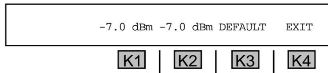
2. Press **K1** to change the low frequency tone level **OR** press **K2** to change the high frequency tone level.
