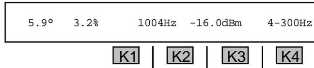
If the readings are relatively the same in the **20-300Hz** test and the **4-300Hz** test, then the source of the excess jitter probably has a fundamental frequency above **20 Hz** since there are no significant contributions to the levels from below **20 Hz**.
