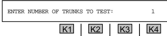
2. If the current parameter displayed is appropriate, press any softkey (**K1-K4**) to proceed **OR** enter a different number of trunks by using the **numeric keypad**.
