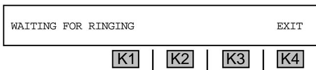
When the **930A** receives ringing it will send the sweep frequencies back. This will continue until the trunk is disconnected (goes back **On Hook**), you exit this display, or a 5 minute time interval has lapsed during which no off-hook supervision has been supplied.
