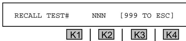
2. Use the **numeric keypad** to input the storage location number (between **00** and **998**) of the desired test setup.
