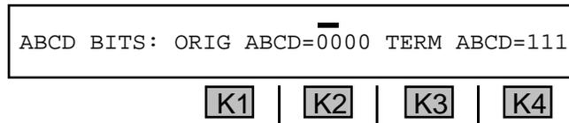
In each of these **T1** span types, the originating end is on-hook. If the **930A** is in **MON1** mode, blanks will be displayed for the **ORIG** side.
