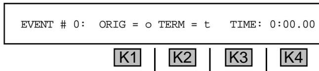
2. Use the **Up/Down Arrow** keys or any softkey (**K1-K4**) to scroll through the list of the results. When you have reached the end of the results, the softkeys and **Up Arrow** key will become inactive. Pressing the **Left Arrow** key will return you to **EVENT #0** and pressing the **Right Arrow** key will advance to the maximum recorded **EVENT #**, skipping all interim events.
