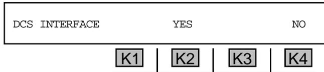
4. Press **K4** under **NO** to exit the **DCS** Interface mode **OR** press **K2** under **YES** to enter the **DCS** Interface mode.
