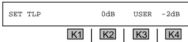
6. Press **K1** to advance the display to the next display without changing any parameters, press **K2** to select **0 dB**, press **K3** under **USER** if you need to set a Send or Receive **TLP** value other than the standard **0** or **-2 dB** values, **OR** press **K4** to select **-2 dB TLP**.
