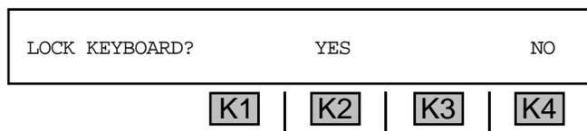
4. Press **K4** under **NO** to discontinue this procedure, **OR** press **K2** under **YES** to lock out all keys on the **930A** front panel.
