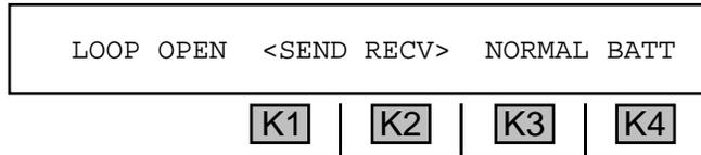
1. Use the **Up/Down Arrow** keys to scroll through the 2 available customer states: **LOOP OPEN** or **LOOPCLOSURE**.
