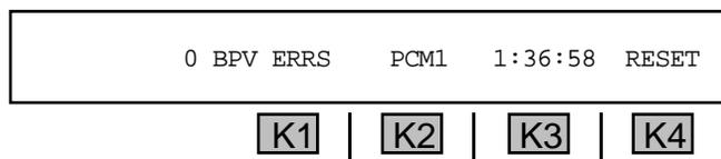
5. Press **K1** or the **Up/Down Arrow** keys to page through the tests described above.
