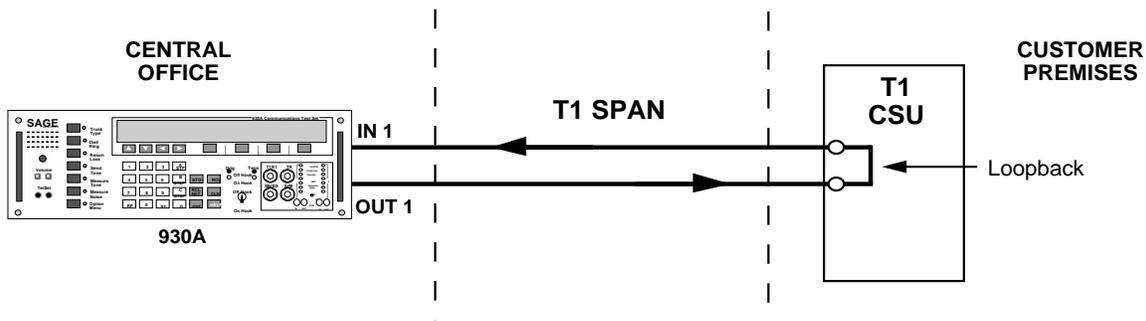
When testing on a T1 facility that terminates into a T1 Channel Service Unit (CSU) on a customers premises, the **930A** can send the **LOOP-UP** code toward the **CSU**. This causes the **CSU** to loop the T1 back toward you.
