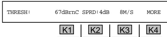
(In **analog** and **wideband**, the Threshold is **54 dBrnC**, in **PCM** it is **67dBrnC**.)
