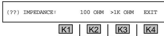
13. Press **K2** to select **100 OHM** impedance or **K3** to select **>1K OHM** impedance.
