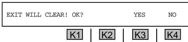
14. Press **K4** under **NO** to resume testing **OR** **K3** under **YES** to end (interrupt). You will be returned to the main display.
