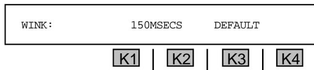
6. Use the **numeric keypad** to change the displayed wink time, **OR** press **K3** under **DEFAULT** to accept the default value. The wink time is the number of milliseconds the **930A** will remain off-hook during a wink.
