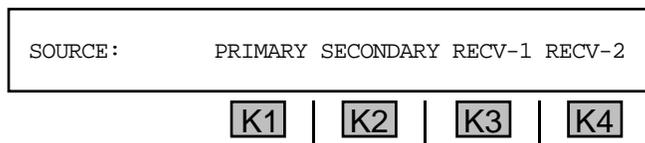
4. Press **K1** or **K2** to view results on the **PRIMARY** or **SECONDARY** channel accordingly. You will be returned to the **RESULTS** display.
