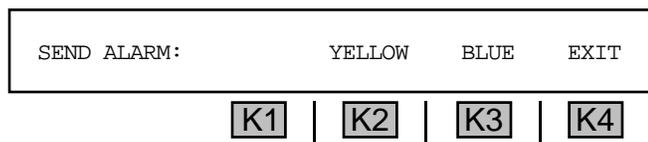
2. Press **K2** to send the Remote (**YELLOW**) Alarm **OR** press **K3** to send the unframed All 1s (**BLUE**) Alarm. When you select an alarm, a cursor appears over your selection.
