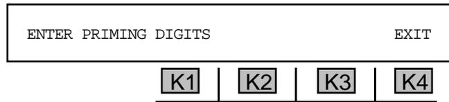
If priming digits had previously been entered, the last string of priming digits will be displayed. If an unwanted string of digits is present, they can be removed by pressing the **CLR** key.
