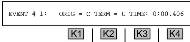
Here the **ORIG** end is off-hook (uppercase **O**) after **406 milliseconds** and the **TERM** side is on-hook (lowercase **'t'**).
