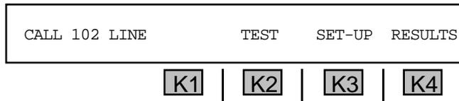
5. Press **K3** under **SET-UP** if you have not previously setup a test. The display reads:
