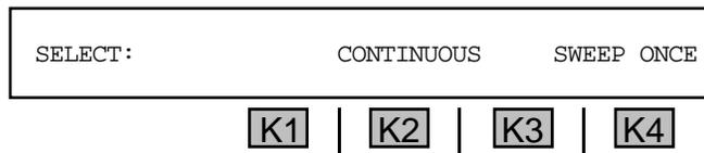
3. Press **K2** under **CONTINUOUS** to continuously repeat the sweep, **OR** press **K4** under **SWEEP ONCE** to sweep only one time. You will immediately hear the sweep tone, and the **930A** will display the expected transmitted or received frequency as the sweep continues. In the **Measure** mode, this is the received level and frequency. The **930A** will display the outgoing frequency and level if it is not in the **Measure** mode.
