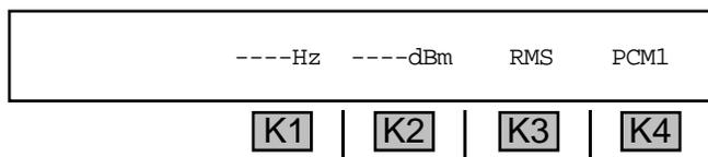
2. Press **K2** once to lock in the current measured value as the **0 dB** reference point. (Pressing **K2** again enables you to input a relative **0** using the **numeric keypad**.)
