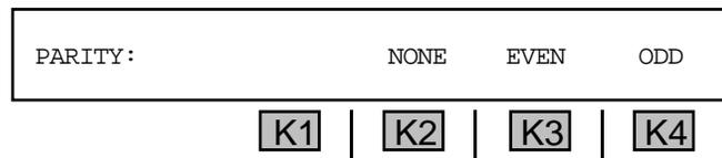
2. Press **K2** under **OFF** for no parity, **K3** for **EVEN** parity **OR** press **K4** for **ODD** parity. The default is **EVEN**. You will be returned to the **SELECT** display after you make your selection.
