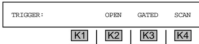
5. Press **K2** to activate **OPEN** mode, press **K3** to activate **GATED** mode **OR** press **K4** under **SCAN** (when in **PCM** mode only) to scan all **24 PCM channels**.
