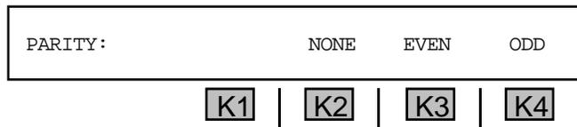
2. Press **K2** under **OFF** for no parity, **K3** for **EVEN** parity **OR** press **K4** for **ODD** parity. The default parity is **EVEN**. You will be returned to the **SELECT** display.
