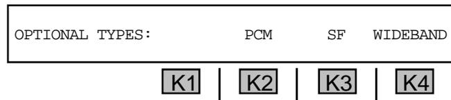
3. Press **K2** under **PCM**. The display below shows the factory default **PCM** display:
