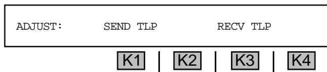
4. Press **K1** under **SEND TLP**. The display shows the current **TLP** setting.
