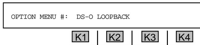
3. Press **ENT** or any softkey (**K1-K4**) to activate your selection. The **LOOPBACK** display reads:
