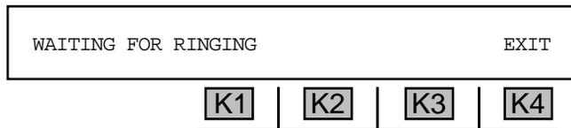
5. If the **930A** is supplying battery or is in **PCM** mode, press **ENT** or any softkey (**K1-K4**) to display the message: **WAITING FOR SEIZURE** or, if the **930A** is in **CONTACT** mode, the display reads: **WAITING FOR RINGING**.
