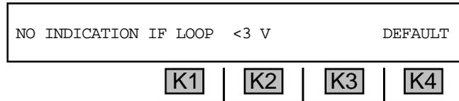
The display above shows that if there is no talk battery present (“dry” loop), there will be no voltage across the loop, and the **930A** will turn off all supervision **LEDs**. This threshold is preset at **3 V**. For this example, this value will be adequate.
