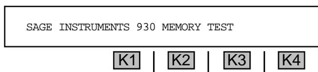
If the memory check is successful the message: **MEMORY TEST** will change to **MEMORY OK!** If the memory test is successful, the display will change to read:
