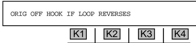
The display above shows the **930A** expecting the battery (Central Office) side of a loop start circuit to provide **-48 V** on **Ring** (2-wire) or **T1R1** (4-wire) in **Normal** mode. In **Loop Reverse**, the **930A** expects to see **-48 VDC** on **Tip** (2-wire) or **TR** (4-wire). It interprets this as the normal on-hook condition. A reversal from **-** to **+** is interpreted as the battery side of the circuit being off-hook. There is no voltage threshold.
