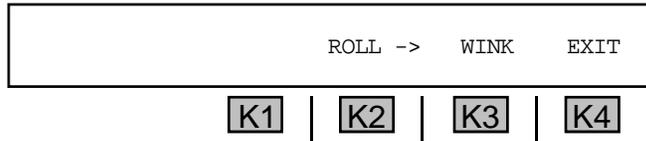
4. Press **K2** under **ROLL ->** to scroll to the next item in the call sequence listed under **K3**. The choices are **WINK, OFF-HK, DELAY, PAUSE, FIXED #, BATCH, TESTLINE** or **DIALTONE**. The **Up/Down Arrow** keys can also be used to scroll through the choices.
