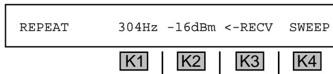
This display shows the level and frequency of the signal being sent to the **Repeat** unit from the **Send** unit. When the sweep completes, the Return Reference part of the measurement is over. It is then followed by the **Repeat** unit sweeping for the Forward Reference test.
