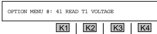
5. Press **ENT** or any softkey (**K1-K4**) to activate your selection. The **930A** will display its readings as Base-to-Peak voltage.
