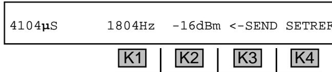
This display shows the calculated phase delay in microseconds for the return reference signal from the **REPEAT** unit, and the level and frequency of the signal being sent from the **SEND** unit. All measurements of **EDD** are made at the **SEND** end of the circuit. **EDD** is also a referenced measurement.
