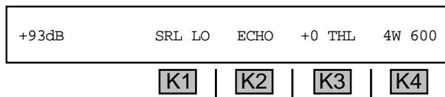
Entering the Return Loss function automatically sets the metallic trunk type to **TERM**. Check or change the **TERM/BRIDGE** setting under the **Trunk Type** function key. (Refer to **Section 3-7.1.**)
