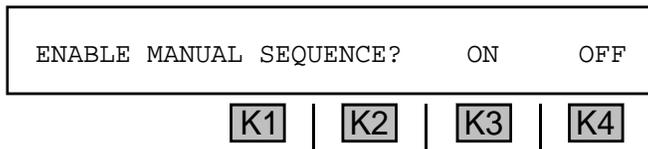
Press **K3** to turn the manual sequence on, but generally the manual sequence is normally **OFF**.
