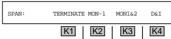
4. Press **K4** under **D&I** to drop the currently selected channel. The other 23 channels pass through undisturbed. Make sure the channel is idle before selecting **D&I**. The display reads:
