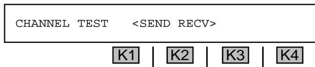
1. Use the **Up/Down Arrow** keys to scroll through the customer states: **CHANNEL TEST, IDLE, FWD DISCONNECT**, or **-R RINGING**.
