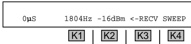
The carrier level should be within the **0 dBm** to **-40 dBm** range and steady for the test to be valid.
