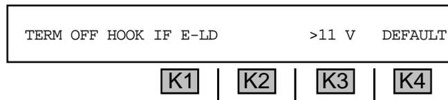
An **Off Hook** indication on the front panel LEDs will be provided if the voltage on the **'E'** lead is below the **11 V** low threshold.
