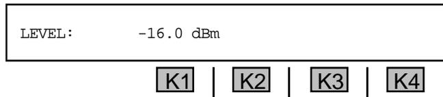
4. Use the **numeric keypad** to enter a new level and then press **K4** under **EXIT** to return to the main **SWEEP** selection display.
