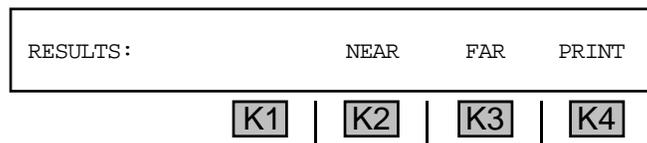
2. Press **K2** under **NEAR** to view the near end results, or **K3** under **FAR** to view the far end results. The first results display reads:
