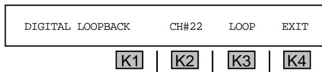
In the above example, Channel 22 (**CH# 22**) has been looped back. You can select a channel between **1** and **24** under **PCM** trunk type. (Refer to **Section 4, PCM Operation** for setup information.)
