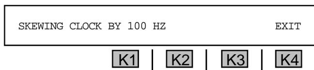
When skew is set properly and the far-end is not loop-timed, a slip will occur *every 2-3 seconds*.
