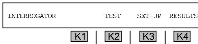
31. Press **K4** under **RESULTS** to see the results of your tests. In **PRINTER** remote mode, the results of each test will be sent to the printer as they occur. In **COMPUTER** remote mode, a bell will be sent to the computer at the conclusion of each test. The test results can be read from the display at that time. (Refer to **Section 6, Remote Control Operation** for more information.)
