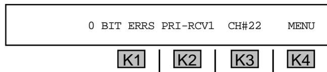
If either **DS0A** or **DS0B** was previously selected from the **CHANNEL** display, the above screen will show the access channel number followed by a colon and the subrate channel. For example, **CH#22:01**. The error results are displayed above **K1**.
