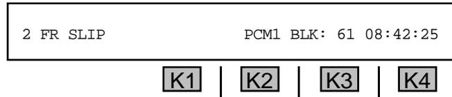
The above display shows the 61st 15-minute block of time since the test began (roughly 15 hours).
